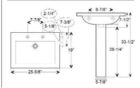
Dimensions of fixture are nominal and may vary within the range of tolerances established by ASME Standard A112.19.2-2018. Dimensions and specifications subject to change without notice.
